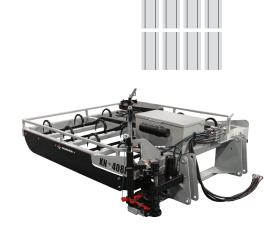
Norden Tie-Grabbers come standard with a single hydraulic circuit. A two-circuit connection is available upon request.
