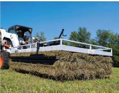
The Kuhns Hay Accumulator system uses gravity and a simple mechanical system to efficiently arrange the bales into a group that is then left in the field. A Kuhns Mfg Grabber or Tie-Grabber mounted on a front end loader or skid steer can pick up the bales and load them onto a waiting truck or wagon. The groups can then be stacked in the barn with a grabber without the operator ever needing to touch a bale.
