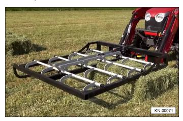
3. Move to the next row of four bales, position the crowd bar against the right side of the row of bales, lower the Grabber onto the bales, and release the bale hooks.
