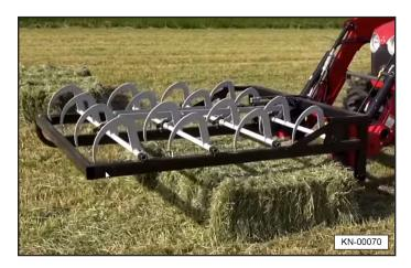
2. Lower the Grabber onto the bales, engage the hooks, and lift the bales.
