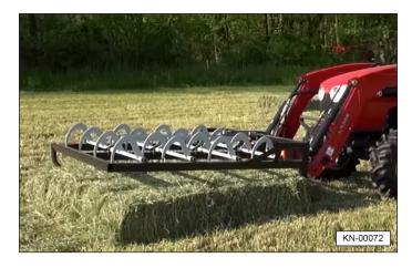
4. Move forward to push the bales together, lower the Grabber onto the bales, engage the hooks, and pick up the eight bale group.
